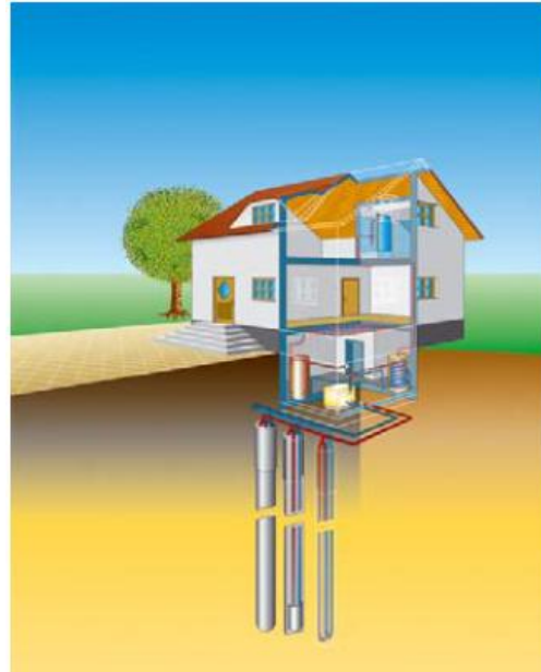
Figure 6. Borehole heat exchangers [13]
