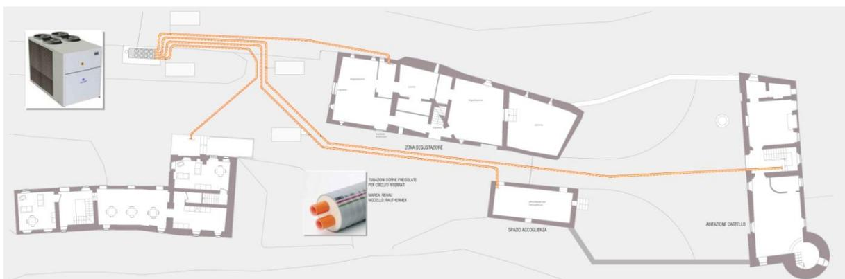
Figure 10. Layout of heating and air-conditioning facilities
