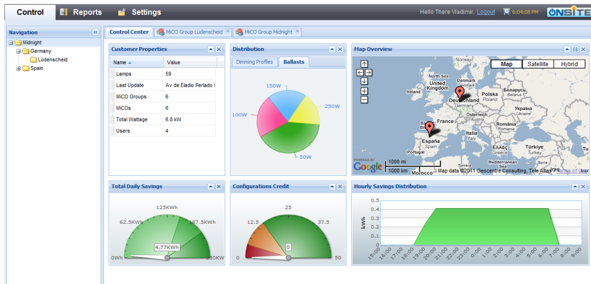
Figure 4. Web link to the MidNight Web application the ON-SiTE, software for programming and street light management
