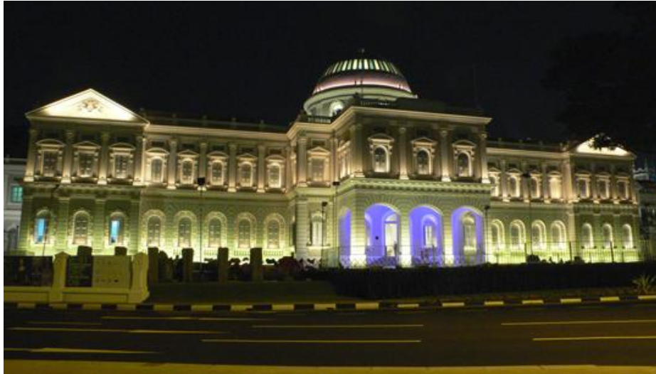
Figure 1. An example of “wall washing” technique
