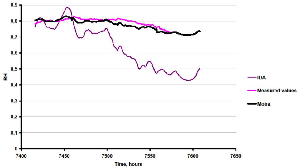
Figure 2. Comparison RH levels of the air in the crawl space for IDA, MOIRA and measured values.
